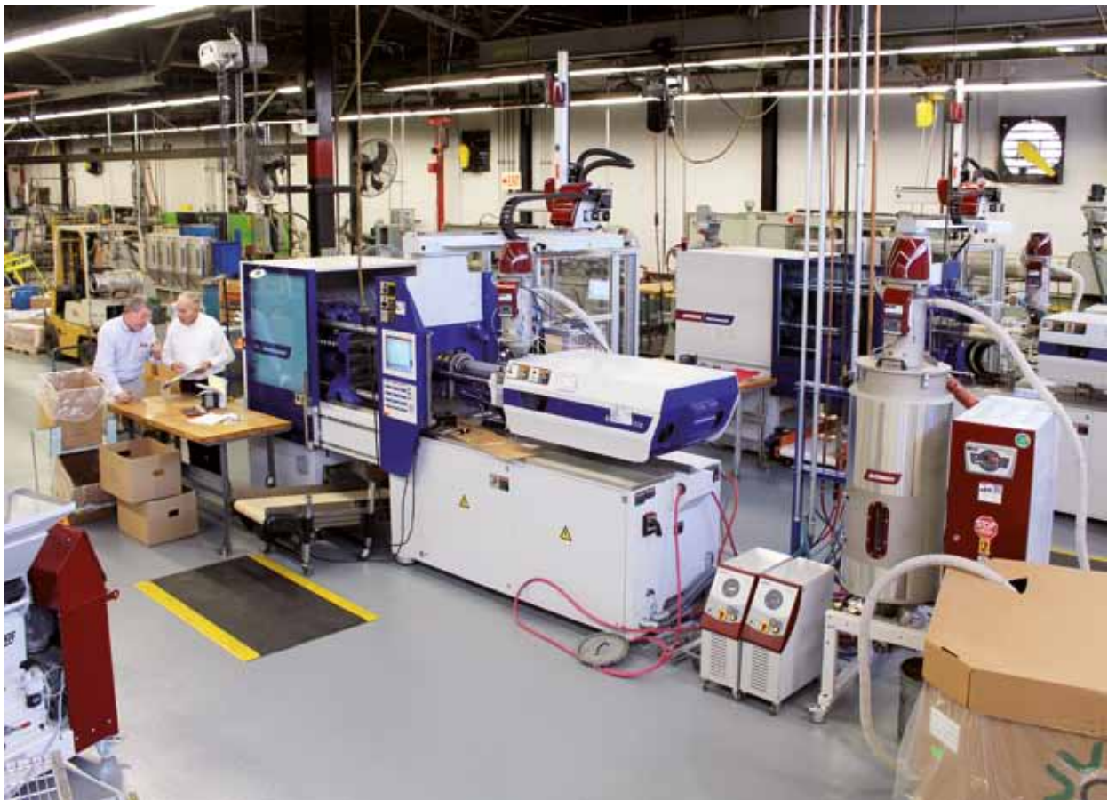
Matt McKenney, Ensinger Precision Components General Manager (left) and Charlie Middelaer stand in front of a WITTMANN BATTENFELD EcoPower 110 injection molding machine, installed at EPC's workflow in Putnam, CT.
