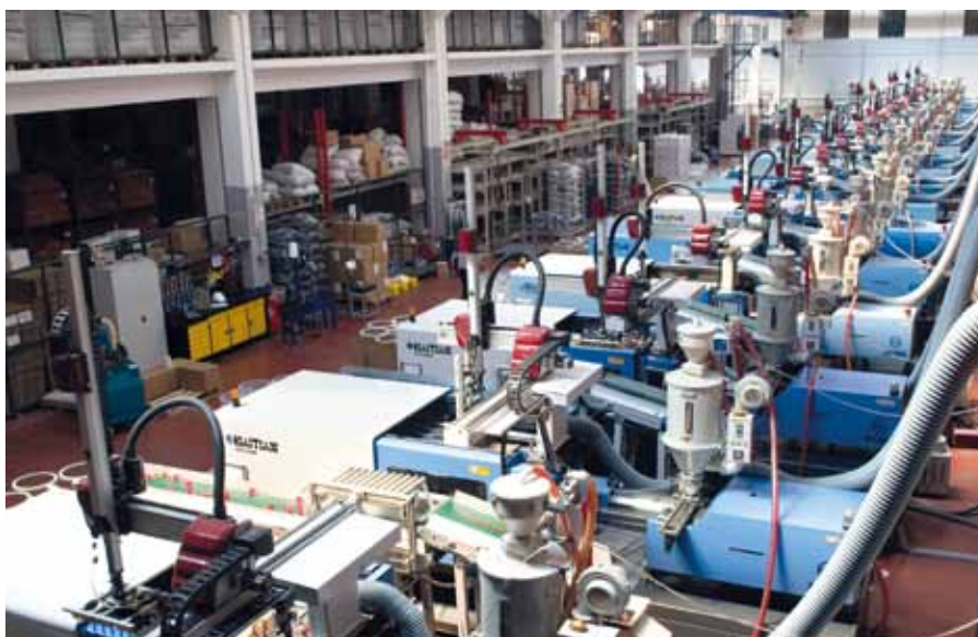
STAR PLASTIK's production hall in Istanbul. All processing machines are equipped with WITTMANN automation systems.
