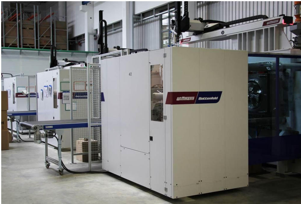
Fig. 1: New production hall at Fröbel in Blaufelden with machines of the PowerSeries from WITTMANN BATTENFELD
