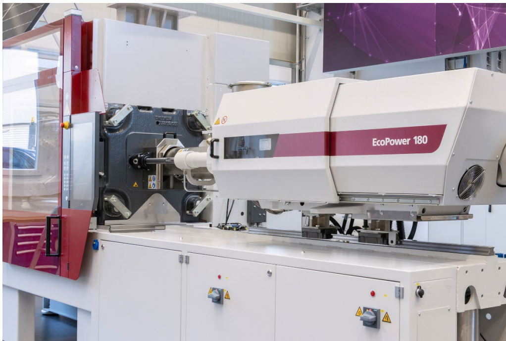
Fig. 3: EcoPower 180/750 with switches for changing between direct and alternating current
