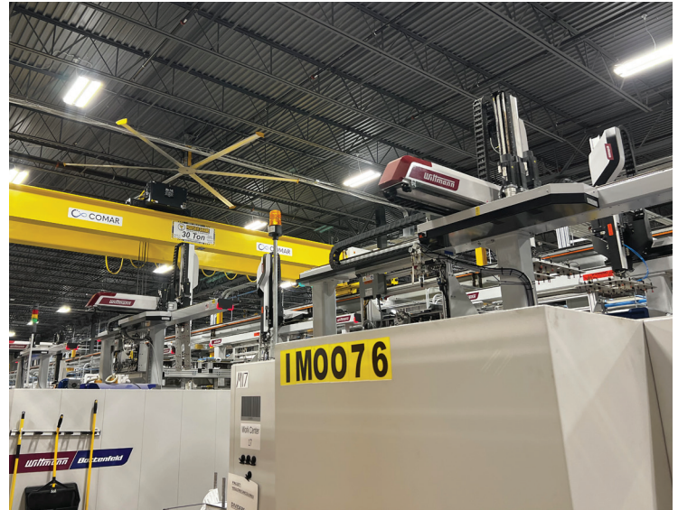
Each of the four new WITTMANN machines at Comar's West Bend plant feature dual high-speed WITTMANN 833 Pro Series Robots
